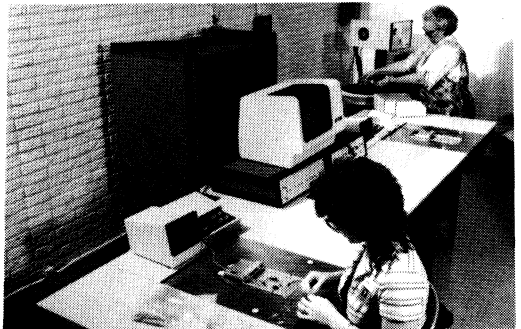
Test fixtures interfaced with Teradyne computer system allows a wide variety of high speed testing programs.
