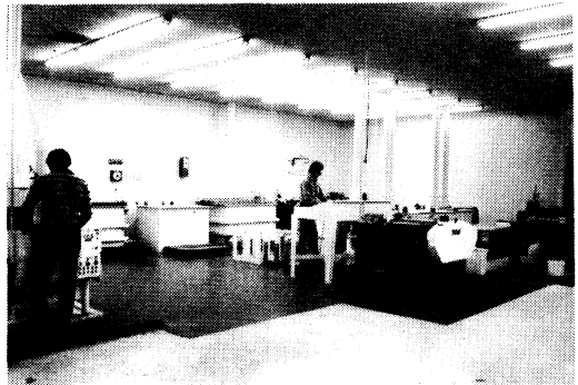
The plating area showing thru-hole plating tanks, reflow soldering, etching, and board washing equipment.
